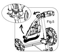
Step 4: Push the red button to rotate the front wheel clockwise 180 degrees to the inner side of the cart as in fig. 4 Step 5: Release the handle buckle, adjust handle to desired position, then tighten the button as in fig. 5
