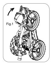
Step1: Adjust the upper bracket to proper position as in fig.1
