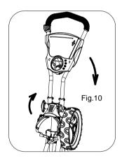
Step 4: Release the upper red button to fold the handle downward then tighten it as in pic 10
