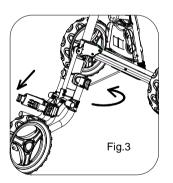
Step 3: Push the front wheel fork downward until the support bracket clicks and then lock the red buckle as in fig. 3
