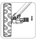
Press the red button on the wheel holder to remove or install the rear wheel.
