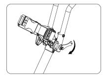
If the handle becomes loose during normal use, please use the supplied tool to tighten the handle as shown above.
