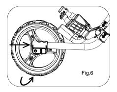
Step 1: Press the red button and rotate the front wheel counterclockwise 180 degrees to outside of the cart as in fig. 6
