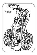
Step2: Unlock the lower red buckle to release front wheel fork as in fig. 2
