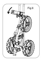
Step 3: Push the upper bag holder bracket downward to the cart folding position as in fig. 9
