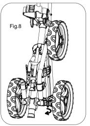
Step 2: Release the lower red buckle, fold the front wheel folk till it click to position. Lock the buckle as in fig. 7 & 8
